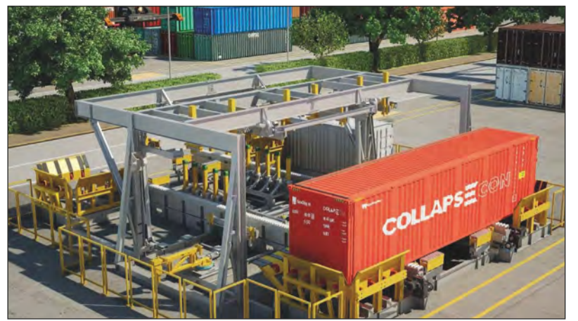
The COLLAPSECON automated operating station, developed by Australia's Spectainer for its horizontally folding container design
