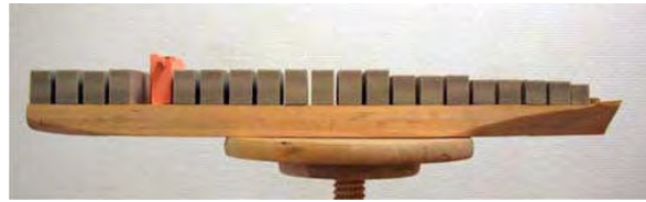
Fig. 1. Full stack configuration of Post-Panamax container ship test model in wind tunnel (Andersen, 2012b).
