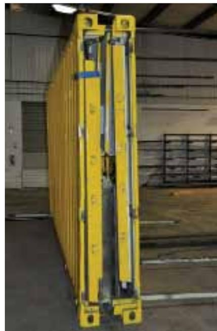
Above and below right: Staxxon containers are foldable, which means empty ones have a smaller footprint and leave more space for full containers.
